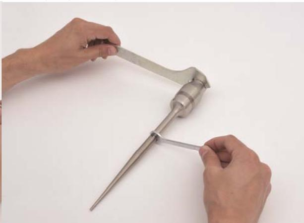
\*Note: When tightening a Microtip, the tip must not be in contact with the work surface. Always have the tip extending off of the table or work surface to minimize stress to the tip.
